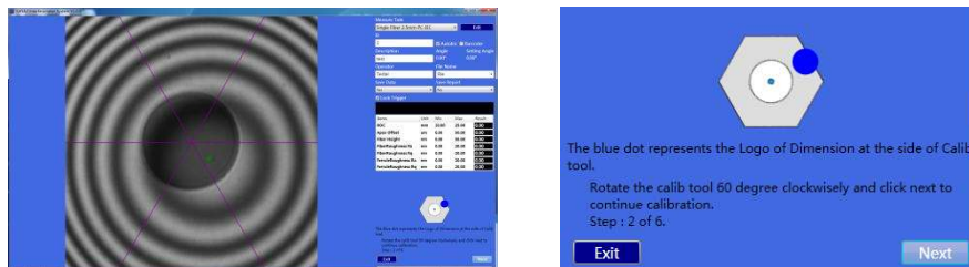
Figure 5- 2 Calibration first step
